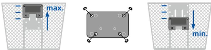
**Mounting** Choose the best basket position with enough space for the light. Insert the nuts into the inner plate and connect the outer adapterplate with 4 screws.
