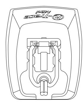
Alternative cable exits: 1. Support pin hole 2. Slot at the bottom
